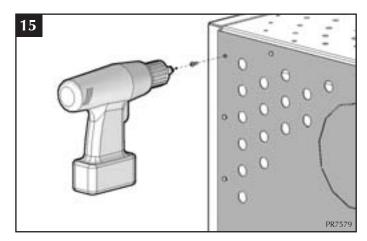
15. Re-attach the back cover plate, internal parts and door.
